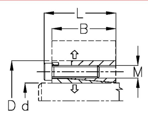
$\begin{array}{lll} \text{B mm} & = 84.0 \\ \text{d H8 mm} & = 280 \\ \text{D mm} & = 355 \\ \text{Fit tolerance} & = \text{Aksel h8, Nav H8} \\ \text{F kN torque} & = 1094 \\ \text{L mm} & = 102 \\ \text{M mm} & = M18 \\ \text{P N/mm2 surface pressure on shaft/hub} = 143 \\ \end{array}$
